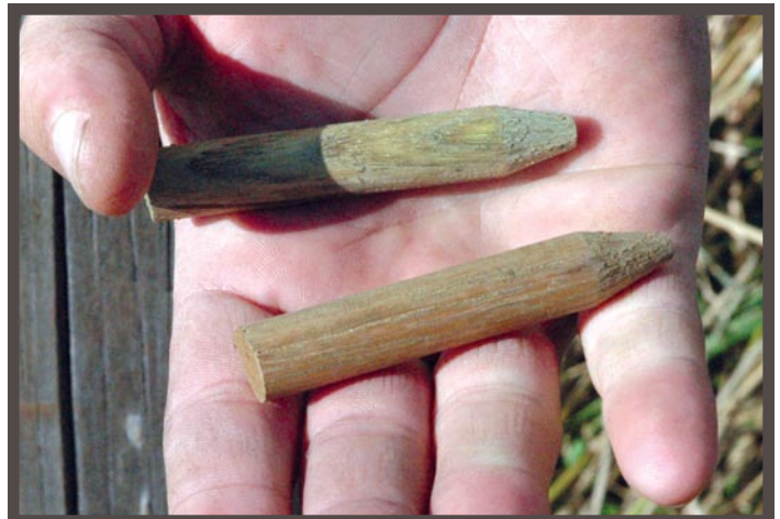
The next step is the bore testing of the pole if indicated. Above: Three bore holes are drilled into the pole to determine if the core of the pole is good and if other problems with the pole exist. Below: Special treated plugs are used to fill the holes left by the boring process. They are hammered in so they are secure.
