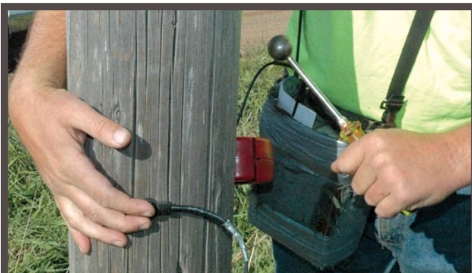
A sonic sounding device is used to determine the health of the pole. This is the second step in pole testing.
